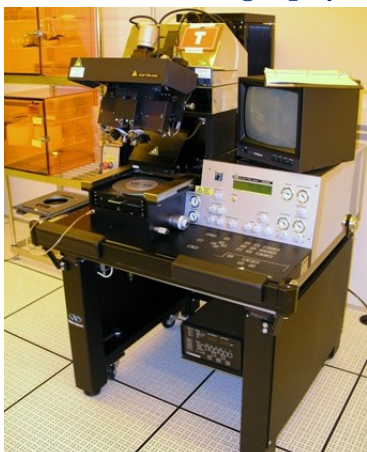
The MA-6 mask aligner exposes photolithographic images on the front and back sides of photoresist-coated substrates up to 150 mm in diameter.
