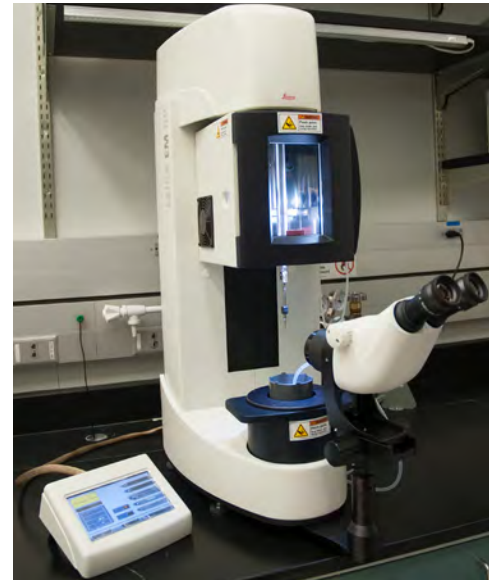
A new automated plunge freezer helps researchers examine nanoparticles and biological specimens in their native state.
