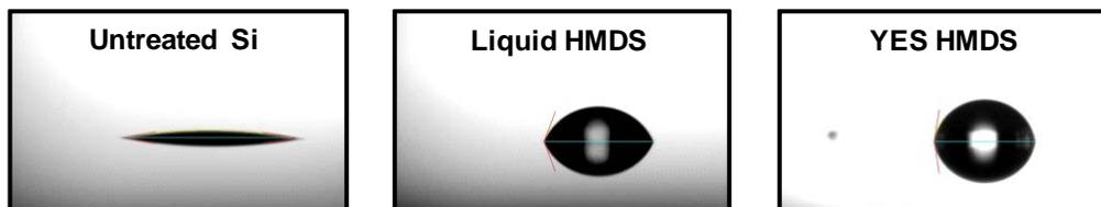
*The wafer contact angle increases with increasing hydrophobicity, with the greatest change achieved using YES HMDS vapor phase priming. The untreated contact angle was 10°; liquid HMDS primed contact angle was 69°; vapor HMDS contact angle was 81°.*
