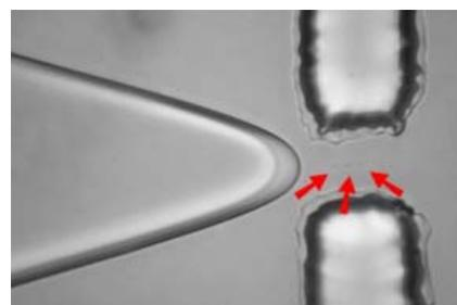
*The NIST “on-demand” single-molecule drop dispenser: Water flows through a microfluidic channel, roughly 35  $\mu\text{m}$  wide, and enters a narrow constriction where it breaks up into droplets (just visible as indicated by the arrows).*
