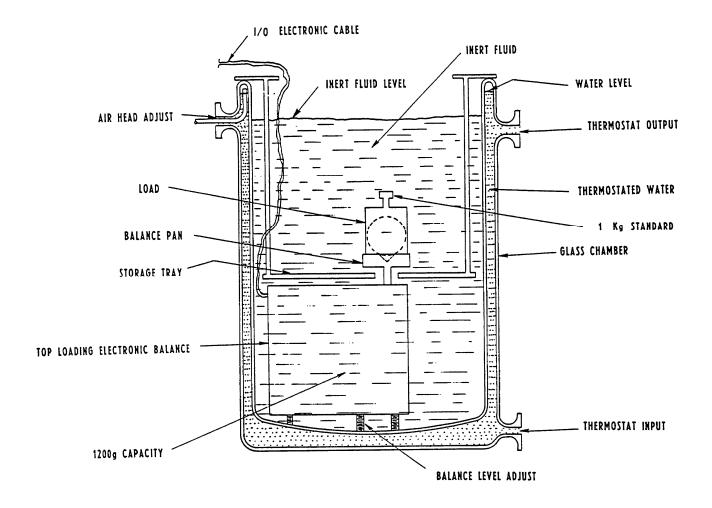
Figure 2. Cross-sectional view of the balance immersed in its thermostated bath. A conventionally-shaped standard weight is shown on the pan. Unconventional loads may also be accommodated by the pan as suggested by the sphere (drawn with dashed lines).
