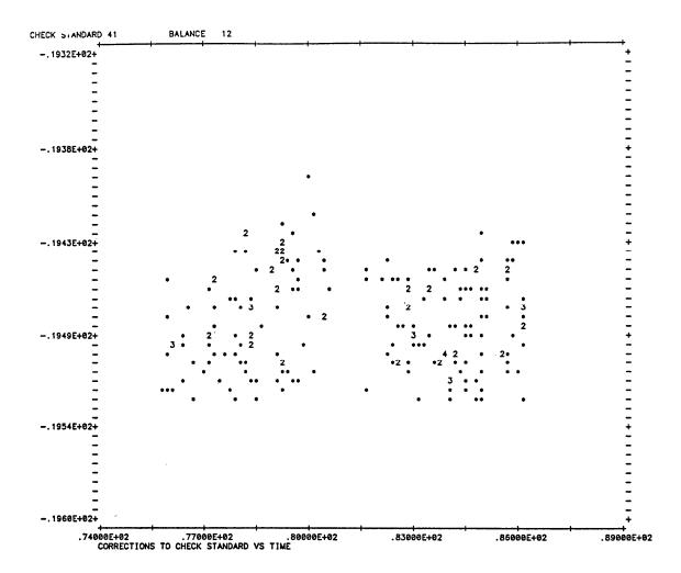
Figure 4. Control chart for the measured difference in mass between kilograms N1 and N2. The ordinate is the difference measured in milligrams and the abscissa is the time of the measurement in years since 1900. Control limits are not shown.
