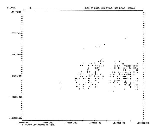
Figure 3. Control chart for the standard deviation of the kilogram balance used in routine mass calibrations. The ordinate gives the measured standard deviation of the balance in milligrams and the abscissa gives the time of the measurement in years since 1900. Control limits are not shown.
