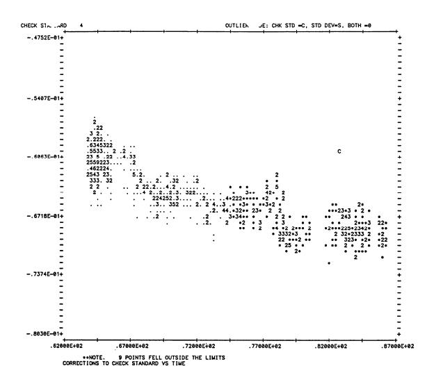
Figure 5. Control chart for the mass of a 1-g check standard. The ordinate is the measured correction to nominal (in milligrams) and the abscissa is the time of the measurement in years since 1900. The check standard is losing mass at the rate of about 0.4 mg/yr. Control limits are not shown.
