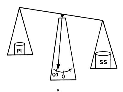
Figure 1. A. A stainless-steel kilogram (density 8000 kg/m $^3$ ) balances a platinum-iridium kilogram (density 21500 kg/m $^3$ ) at normal atmospheric conditions. B. Under vacuum conditions one can see that the mass of the stainless-steel kilogram actually exceeds that of the platinum kilogram by about 0.1 g.
