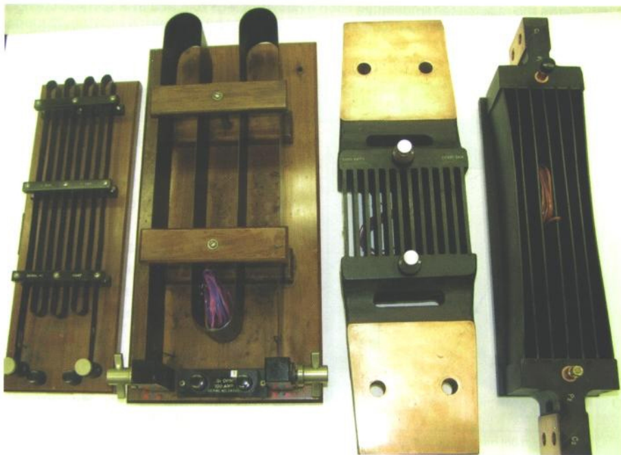
Figure 2. Shown from left to right are a 0.1 \Omega / 15 A ribbon shunt, a 0.01 \Omega / 100 A ribbon shunt, a 10 \mu\Omega / 3000 A parallel element shunt, and a 100 \mu\Omega / 1000 A parallel element shunt.
