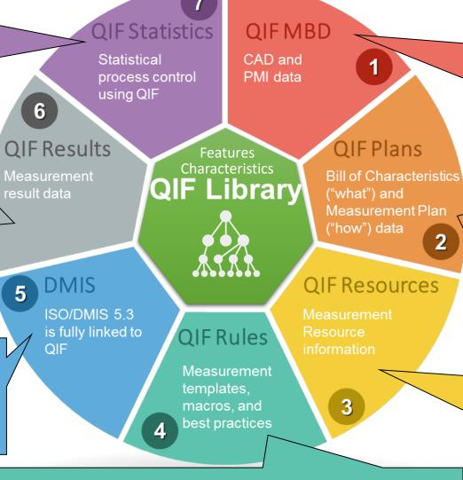
Create measurement rule templates. (e.g., *If a Surface Profile tolerance value is less than* **x**, *then use a CMM method with at least* **y** *number of point/sq.in.*) QIF MBD is the base for providing traceability to authority CAD data. It is not required for basic QIF use cases. Considered to be the strongest semantic CAD+PMI standard available.
