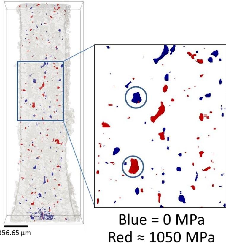
In-situ XCT mechanical testing, showing pores under zero load and 1050 MPa (past yield) in AM IN718 (Kafka, ICAM, 2021)
